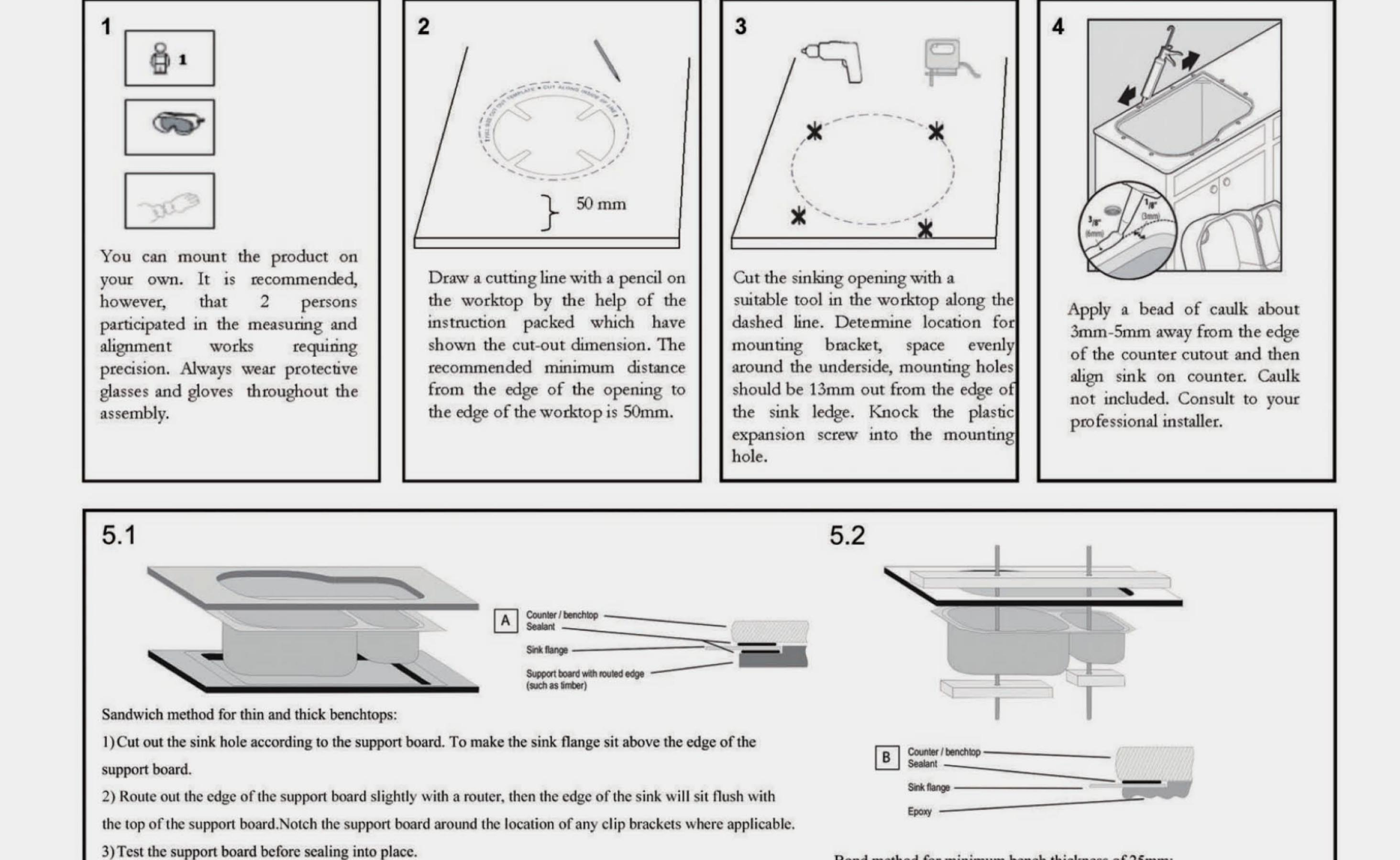
4) Install sink and seal between flange of sink and support board.
